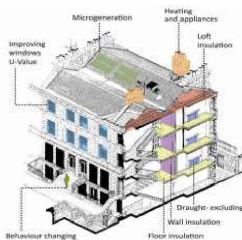
Fig. 6 B. A range of measures can be applied to a traditional Edinburgh tenement but critical to them is behavior change
